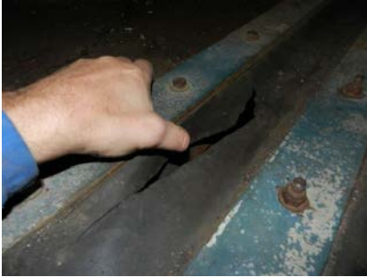
Failing inner cab roof seal leading to ineffective cab ventilation exacerbated by a cramped cab
